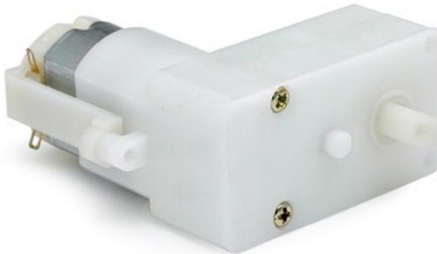
The two small geared motors (unfortunately the Xbox vibration motors were not powerful enough) need connected to the PWM motor output connectors.
